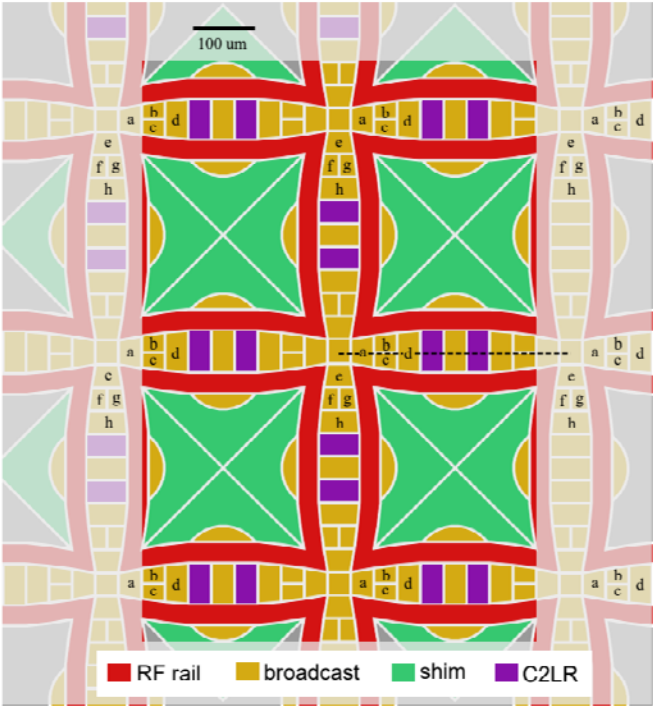
FIG. 1. Representative drawing of the top metal detailing the rf rail (red), generic control electrodes (yellow), special center-to-left-or-right electrodes (C2LR, shown in purple), shim electrodes (green), and ground plane (gray). The rf rail is continuous; the apparently isolated top metal features are connected through traces routed beneath the surface [10] The generic control electrodes are co-wired between equivalent locations in each leg. Lettering on several such electrodes illustrates the pattern. All measurements here use legs in the 3 \times 2 region at the center of the grid (bold).
